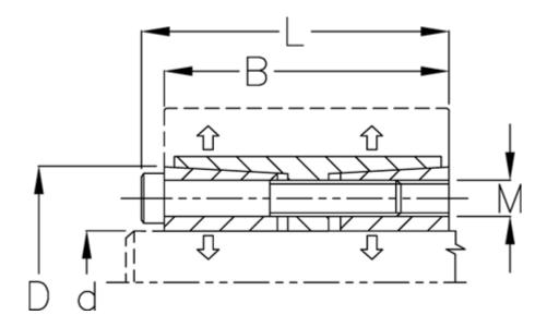
B mm = 155d H8 mm = 420D mm = 515Fit tolerance = Aksel h8, Nav H8 F kN torque = 3343.0L mm = 177M mm = M22P N/mm2 surface pressure on shaft/hub = 150 Surface roughness = R? ?  $3.2 \mu n$ T N m torque = 702000Ts N m bolt tightening torque = 930.0
